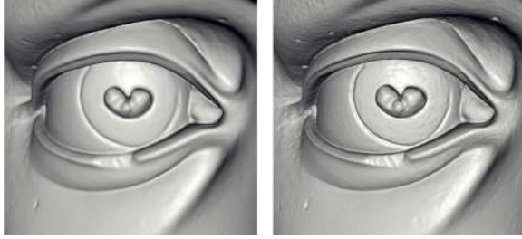
Figure 4: Comparing the results of the in-core algorithm (left; h=11 ; 4,442 MB peak memory) and streaming algorithm (right; h=13 ; 780 MB peak memory).
