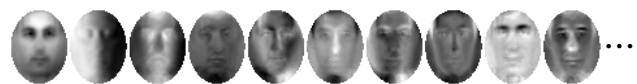
Figure 3: \mathbf{U}_{\text{pixels}} contains the PCA eigenvectors (eigenfaces), which are the principal axes of variation across all images.
