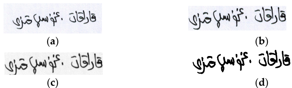
Figure 3. Preprocessing signature image: (a) initial image; (b) normalization image; (c) denoise image; (d) binary image.
