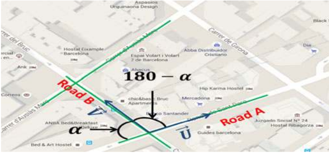
Fig. 3. The \alpha parameter to detect if two vehicles are in line of sight or not.
