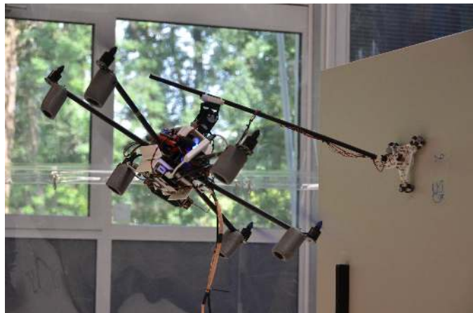
Fig. 1: Photo demonstrating the multimodal locomotion system performing a cleaning operation on a vertical surface.
