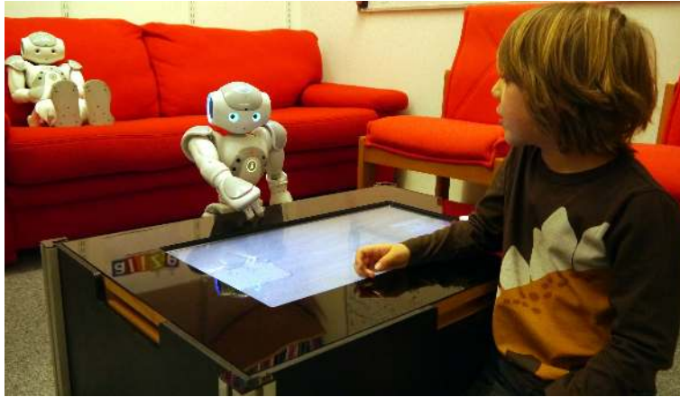
Figure 3. The ‘SandTray’ setup: social interaction between robot and child is facilitated by a touchscreen, which provides a collaborative activity where they can equally participate.
