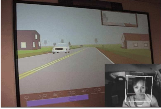
Figure 2: Audio-visual platform installed in a car simulator. The face of the driver is tracked using a camera installed near the rear view mirror: the white cube surrounding the driver’s face corresponds to \Pi , the location and orientation of the pose estimate.
