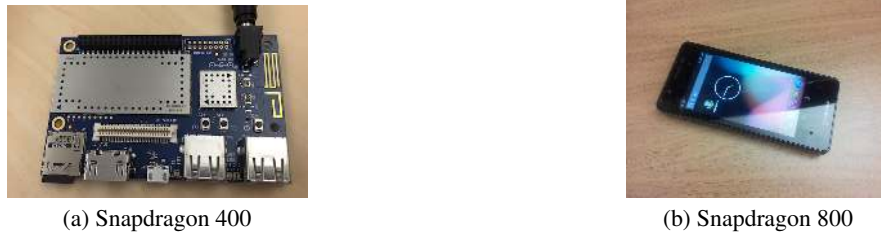
Fig. 12. The development board for profiled wearable-class hardware; processors and measured energy profiles of the boards are identical to that of processors found in commercial wearables. For example, the Snapdragon 400 (a) is found within smartwatches, such as the LG G Watch R Smartwatch and (b) Snapdragon 800 is found within Samsung Galaxy 9005 and Nokia Lumia 1520.
