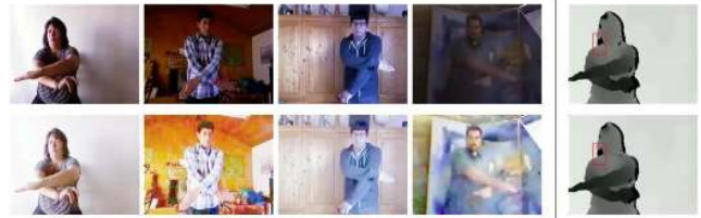
Figure 2. An example of our video enhancement on RGB (left part) and depth (right part) data. The first row represents videos without pre-processing. It is obvious that the illumination of RGB videos with different performers can vary a lot. The depth videos mainly suffer from noises along with edges. Retinex is processed on RGB and median filter on depth videos. The result on the second row shows our strategy is effective to enhance both videos.
