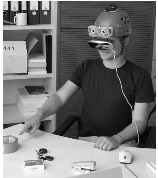
Figure 1: User with head mounted cameras and display. The input is looped back into the display and enhanced by visual augmentations.
