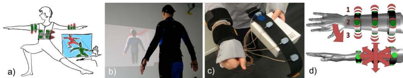
Figure 1: a) Multimodal feedback guides a user to follow directed motion from a remote teacher. b) Motion capture allows full-body feedback. c) Vibrotactor hardware d) for continuous feedback on speed and direction.
