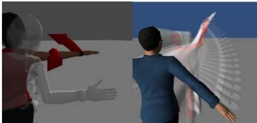
Figure 7: (Left) Motion guidance using ghost avatar and directional arrows. (Right) Motion sequence with transparent avatars, where the red avatar indicate a compulsory pose.
