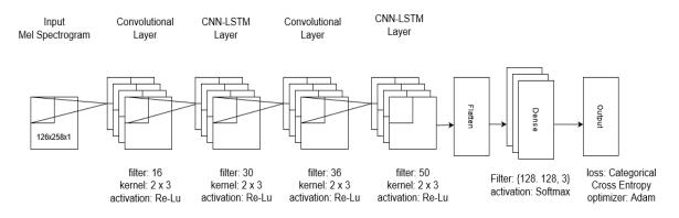
Figure 2. The architecture of the proposed CNN-LSTM
