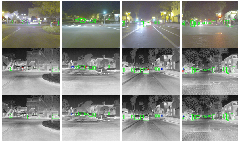
Fig. 17. Qualitative results on more testing examples in FLIR dataset. We place RGB-thermal images in triplet: in each macro row (divided by the black line), we show RGB images in the upper row and thermal images in two lower rows. Over RGB images, we overlay ground-truth annotations, highlighting that RGB and thermal images are strongly unaligned. To avoid clutter, we do not mark class labels for the bounding boxes. On the thermal images, we show detection results from our thermal-only (mid-row) and best-performing ProbEn (with bounding box fusion) model (bottom-row). Green , red and blue boxes stand for true positives , false negative (mis-detected persons) and false positives .
