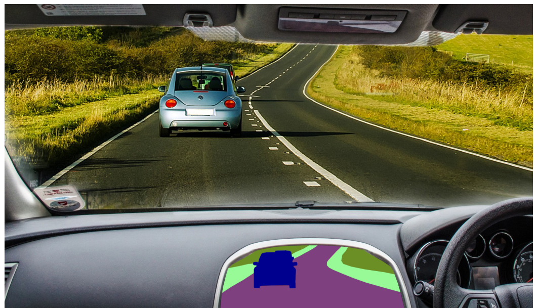
Figure 1. The car screen shows an example of semantic segmentation of the scene in front of the car.
