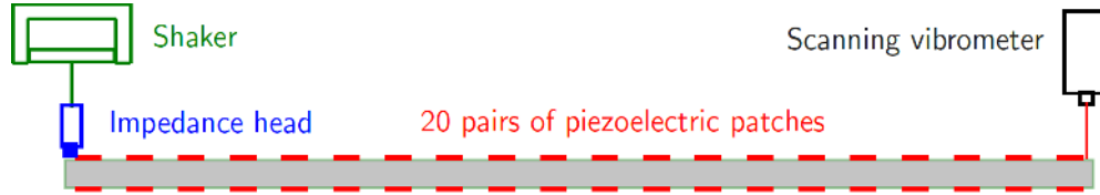
Figure 10. Experimental setup for the analysis of transverse waves.
