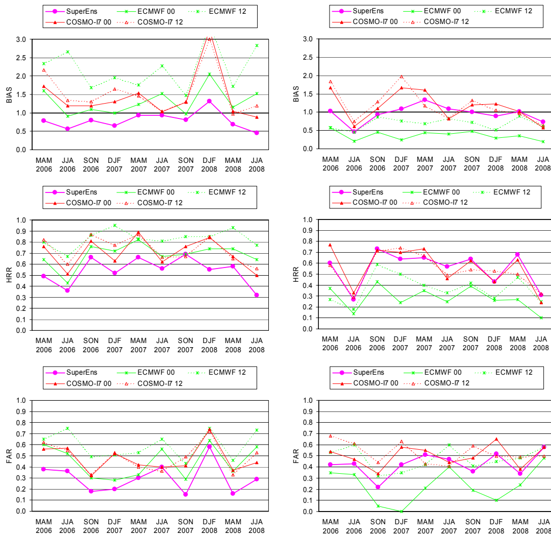
Fig. 9. Verification indices for Multimodel SuperEnsemble ECMWF IFS 00:00 UTC and 12:00 UTC, and COSMO-I7 00:00 UTC and 12:00 UTC runs for +12h+36h forecasts. Average values, threshold 10 mm (left) and maximum values, threshold 35 mm (right) BIAS, HRR and FAR.
