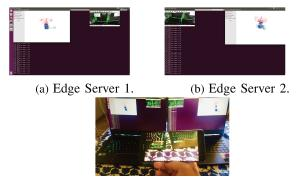
(c) Simulatneous mobile client offloading to two edge servers. Both servers maintain a map of the environment (a and b). The application combines both maps and displays it (c).
