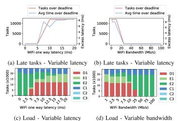
Fig. 10: Impact of WiFi latency and bandwidth on task allocation and excess latency. For latencies > 5 ms, in-time completion rate drops to 50%. Minimum completion rate is achieved for bandwidth > 25 Mb/s
