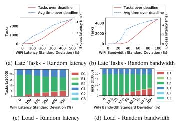
Fig. 12: Impact of WiFi latency and bandwidth standard deviation on task allocation and excess latency. The system can withstand up to 100% stdev for bandwidth and 25% stdev for bandwidth until late tasks happen.
