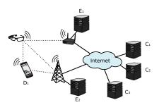
Fig. 3: Environment model: a pair of smartglasses is connected to several computing units located at different extremities of the network: device to device  $(D_k)$ , edge  $(E_k)$  and cloud  $(C_k)$ .
