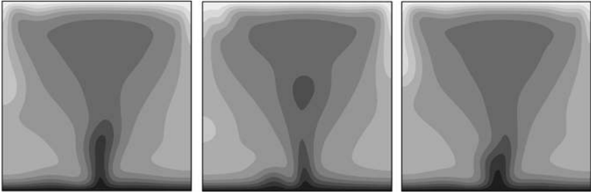
Figure 5. Oscillatory convection at Ra_{th} 800. The evolution of the normalized temperature T is shown at three different time-steps for one oscillatory cycle. Small convection cells shear off at the bottom boundary at a characteristic dimensionless frequency of 270 and merge with the main plume in the center. At Ra=800 , other studies reported dimensionless frequencies of 280 (Kimura et al. , 1986), 296 (Caltagirone and Fabrie, 1989), 299.7 (Cherkaoui and Wilcock, 1999), and 287.2 (Schoofs, 1999). Contour levels are in 0.1 intervals from 0.0 to 1.0.
