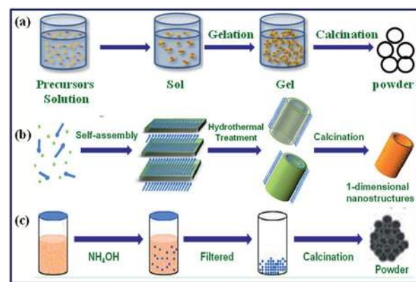
Scheme 2 Schematic representation of the chemical synthesis routes of SMON via (a) sol-gel, (b) hydrothermal, and (c) co-precipitation methods 8 Reprinted with permission from ref. 8. Copyright 2016, DRDO.
