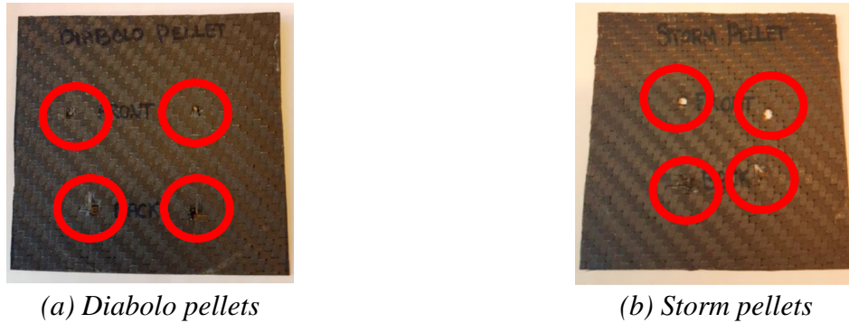
Figure 8-Visual inspection of the impact
