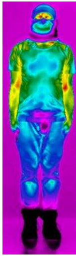
(I) Outside cold room (a) Subject is wearing jeans, t-shirt, underwear, surface temperature without additional clothing ( T_s (°C))
