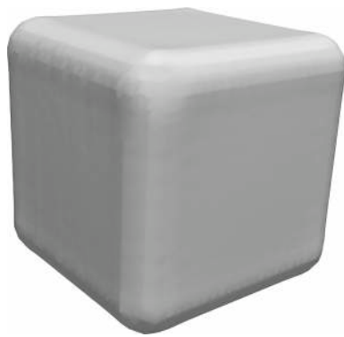
Fig. 8 Unit cube, zero iso surface of the radial basis function used to describe the cube boundaries for the imposition of constraints
