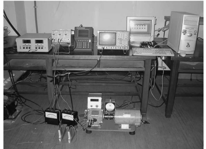
Fig. 3. Actual experiment setup to collect the healthy and faulty motor data.
