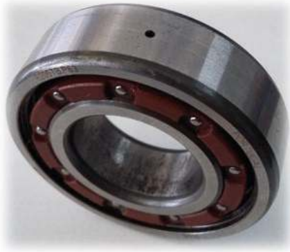
FIGURE 5: Outer race damaged bearing.
