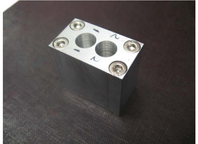
Fig. 11. A drilled 2-horn array prototype.
