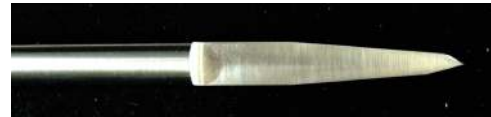
Fig. 5. The machine tool used for the fabrication of the drilled horn prototype.
