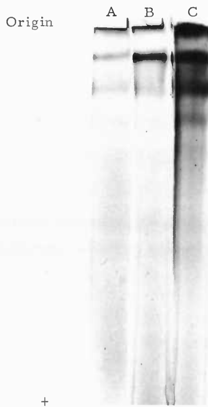
Figure 16. Electrophoretic pattern of fractions: A, CM_I ; B, CM_{II} ; and C, unfractionated S_I . \alpha -Naphthyl acetate was the substrate.
