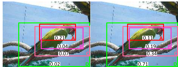
Figure 1. Detection results without/with classifier refinement (left/right). Detection scores are plotted in the bottom of the sampled proposals A, B, C, and D. In the left, the top ranking proposal A does not correctly localize the object. After instance classifier refinement, in the right, the correct proposal D is detected and more discriminative performance of instance classifier is shown.
