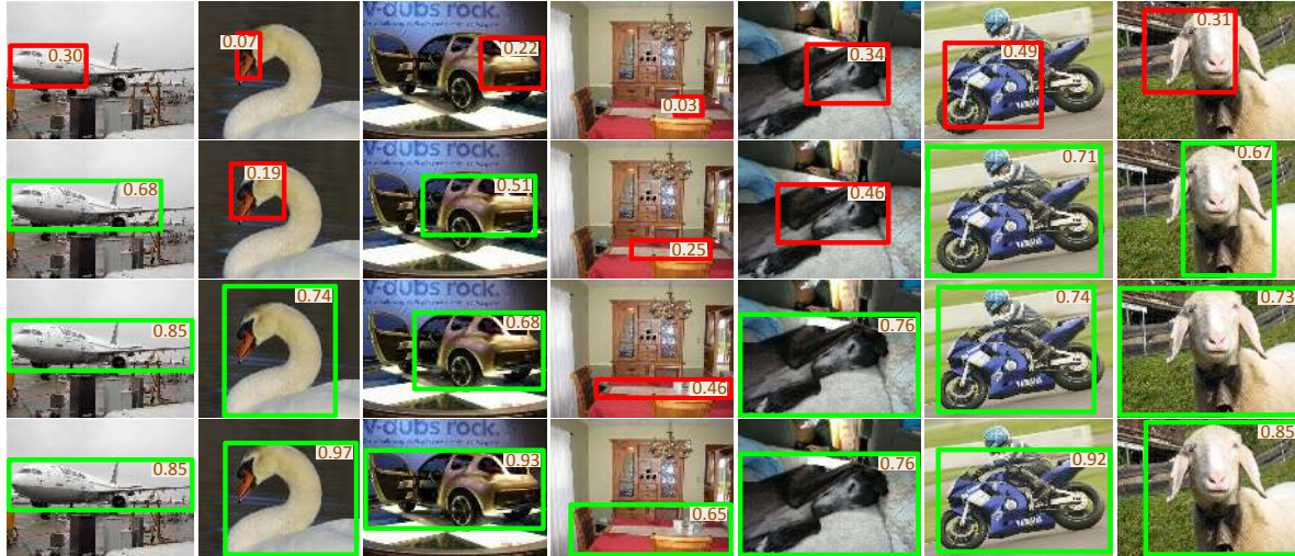
Figure 2. Detection results from different stages of classifier refinement. Each row represents one stage. Green/red rectangles indicate detected boxes having high/low overlap with ground truths, and digits in the top right corner of rectangles indicate the IoU. Through multi-stage refinement, the detector can cover the whole object instead of parts gradually.
