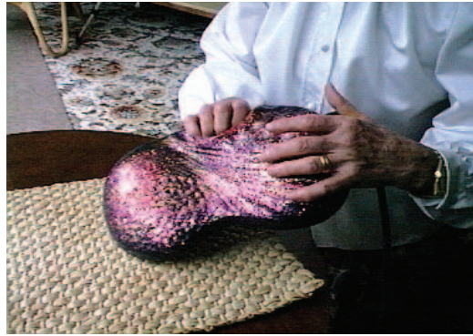
Figure 1. The shell instrument, which is responsive to touch. The instrument is a fiberglass mold set in transparent resin, in which piezoelectric sensors are embedded.
