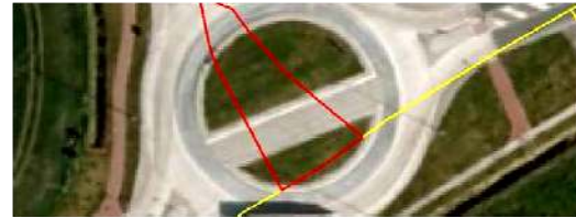
Figure 6: Redeveloped roundabout identified by grassland detection (revised roads = red, no decision = yellow)
