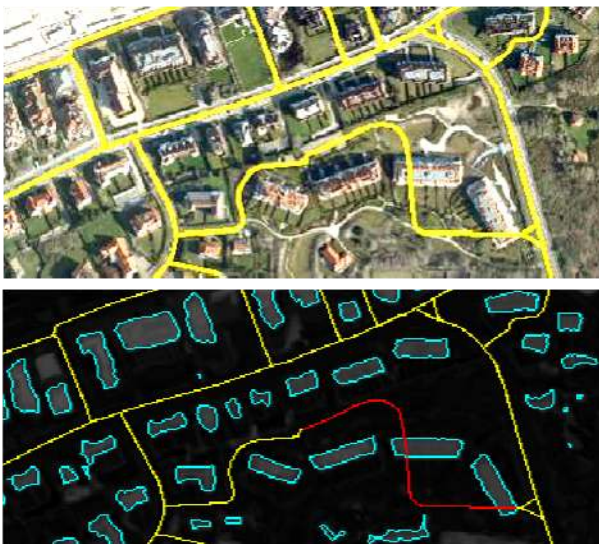
Figure 5: Building module. Top: image superimposed with database roads containing one incorrect object. Bottom: nDSM superimposed with extracted buildings (cyan) and evaluation result (incorrect = red, no decision = yellow)
