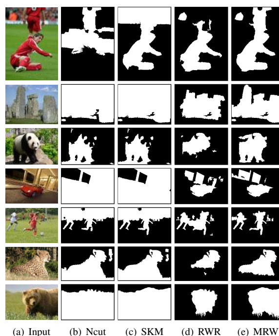
Figure 3. Bilayer segmentation results of the proposed MRW clustering in comparison with the conventional approaches: Ncut [26], SKM [21], and RWR. In the RWR results, the initial distributions based on the center prior are used as the fixed restart distributions.
