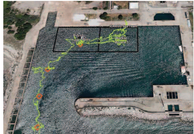
Fig. 9 – MARES AUV autonomous navigation trajectory (with required resurfacing waypoints and detected underwater targets location).
