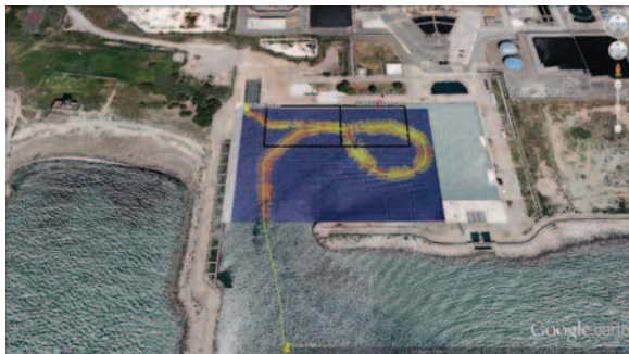
Fig. 5 – ROAZ trajectory and single pass realtime bathymetry survey along path superimposed in Google earth.
