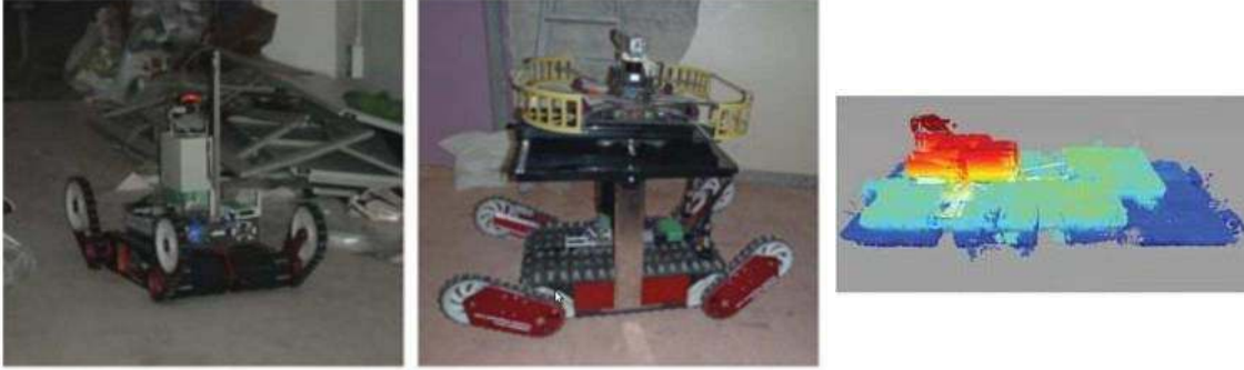
Figure 8: Heterogeneous robots used to map an earthquake-damaged building: (left) Kenaf ground robot, (middle) Quince ground robot and a Pelican quadrotor. Kenaf and Pelican are equipped with scanning laser rangefinders. Quince transports Pelican from one site to another. (right) A sample 3D map of three floors, developed using scanning laser rangefinders of Kenaf and Pelican. Image courtesy of Nathan Michael et al. (Michael et al., 2012).
