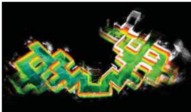
Figure 14: A 3D map developed by laser ranger measurements using GraphSLAM. Image courtesy of Keiji Nagatani et al. (Nagatani et al., 2011).
