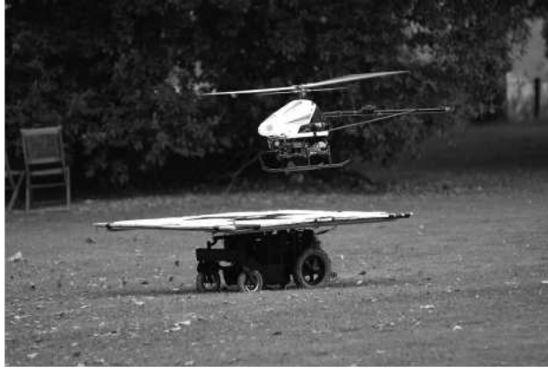
Figure 7: Using line-of-sight observations, a rotary wing UAV lands on a moving platform autonomously. Image courtesy of Thomas Richardson et al. (Richardson et al., 2013).
