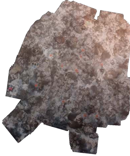
Figure 22: Map of an underwater environment, developed by two robots using feature-based image registration. Image courtesy of Armagan Elibol et al. (Elibol et al., 2014).
