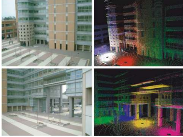
Figure 17: Examples of 3D maps of outdoor environments using the cooperative positioning system. Image courtesy of Yukihiro Tobata et al. (Tobata et al., 2012).
