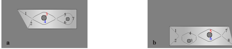
Figure 25: Two partial maps of the same environment with their probabilistic GVDs. There is a displacement between the maps. a) PGVD of the first map. b) PGVD of the second map (Saeedi et al., 2014a).
