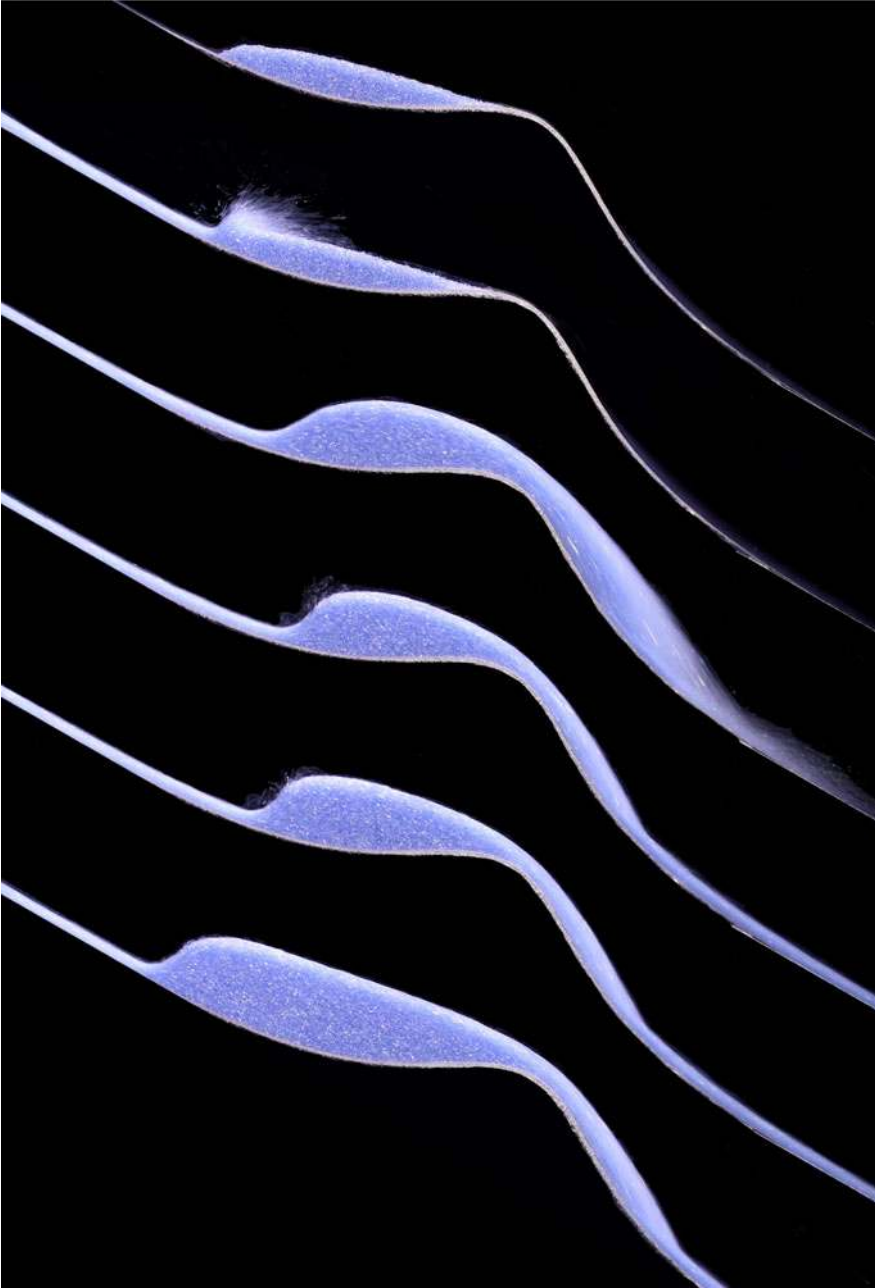
FIGURE 2. Snapshots of an experiment showing the time-dependent evolution of the shock towards steady state. As the oncoming material from the inflow collides with the layer of static particles upstream of the bump there is a sharp decrease in bulk velocity and associated increase in flow thickness. This shock propagates upstream until it reaches an equilibrium position. The experiment is performed at a constant slope angle \theta = 39^\circ with pictures taken at times t = 0; 0.4; 0.7; 1.0; 1.5 and 4.0 s. Note that the images have been slightly rotated to maximise space. The bump height of 4.75 cm acts as a scale. A supplementary movie is available online.
