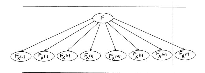
Using the binary partition (as suggested by (1)) and choosing the same variable for splitting at the next two levels, we get the binary tree shown below:
