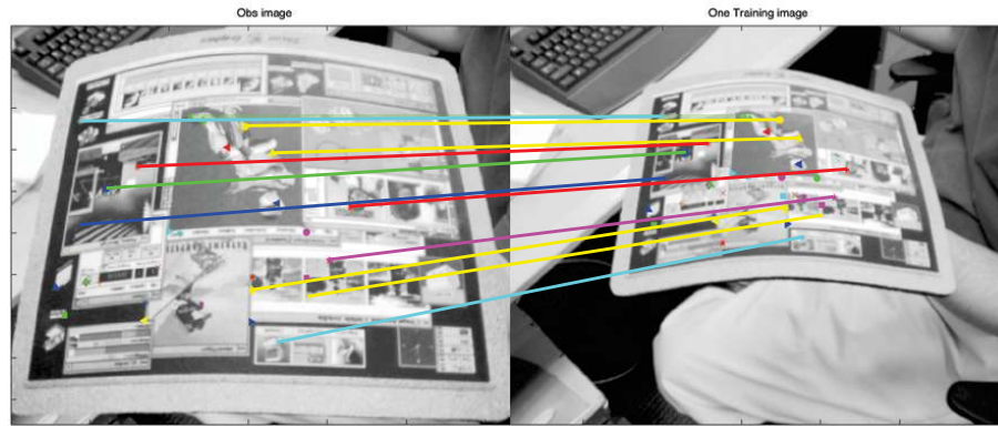
Fig. 3. Translational + KPCCA: Matching using a non-planar surface undergoing warping and scale changes. During training, the object was moved away from the camera and deformed. (Left) shows the first image of the training sequence. (Right) shows the test image, which is outside of the training sequence. The shapes and colors indicate the corresponding points. In this example, 50 feature locations were correctly matched, with 10 false positives. Some lines between matches are included for clarity.
