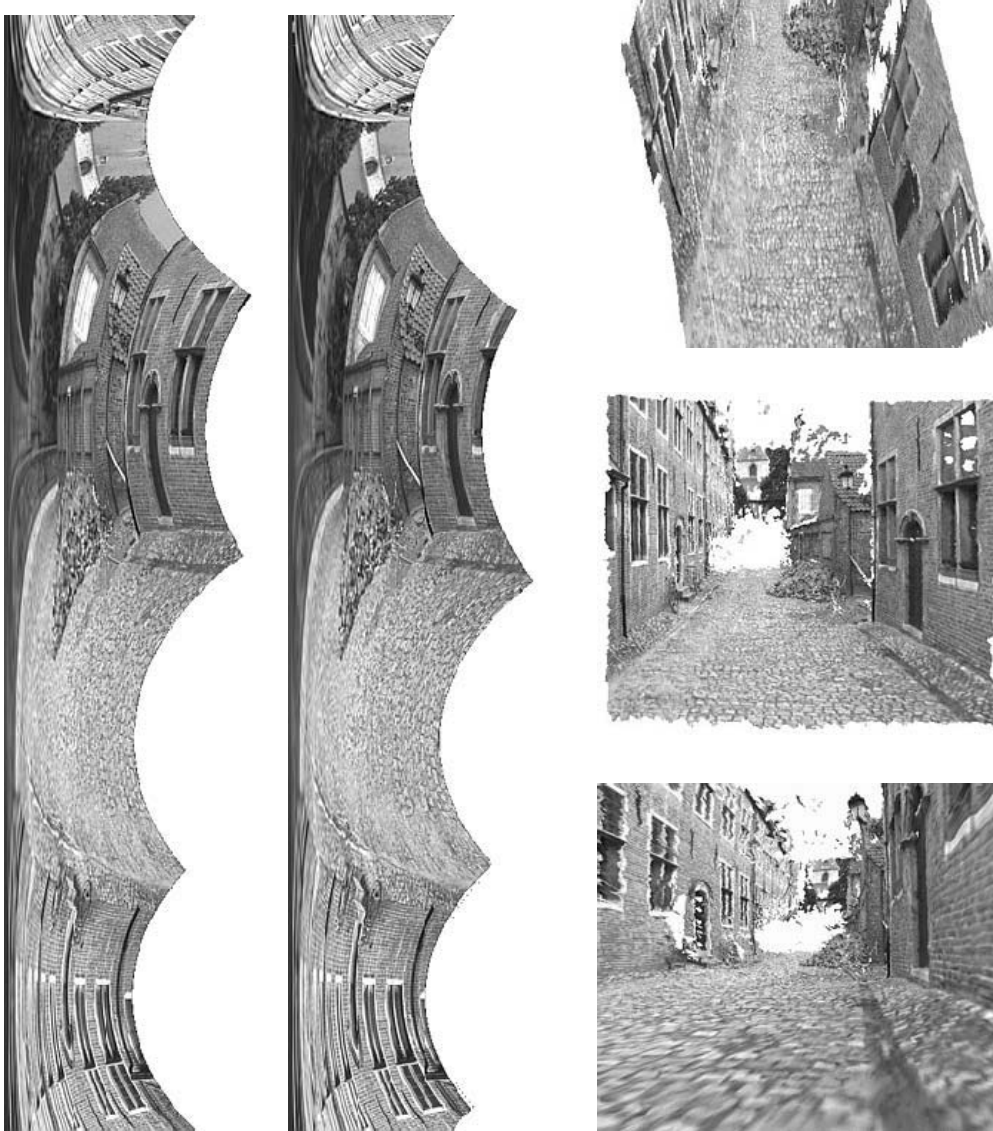
Figure 3.16. Rectified image pair (left) and some views of the reconstructed scene (right).
