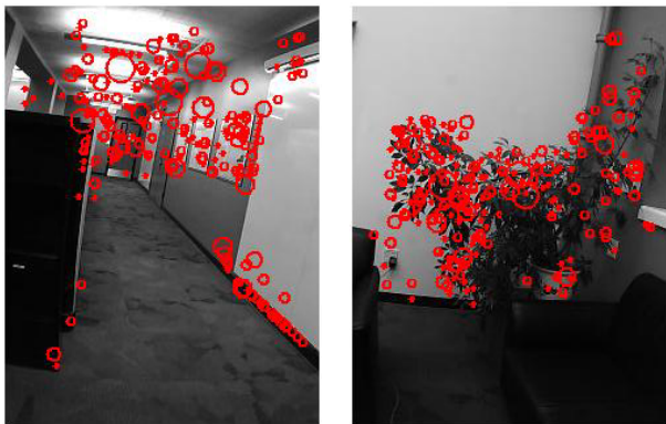
Fig. 4. The interest points detected from a corridor scene (left) and a tree object (right). The SURF features are superimposed as red circles.
