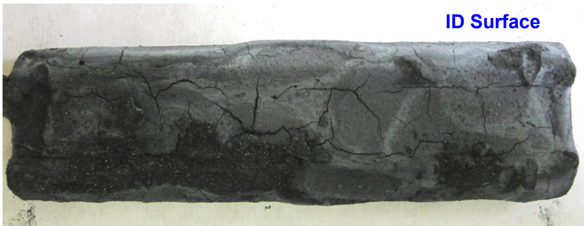
Figure 4. The typical views of the test specimen (ID and OD surfaces) after the ash deposit coating (prior to the corrosion testing) are shown.
