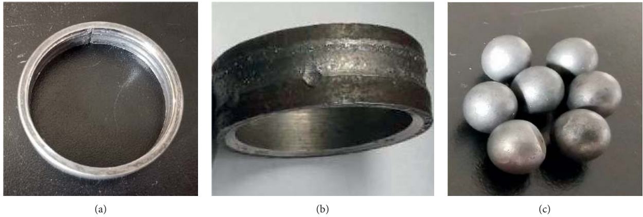
FIGURE 13: Different fault types of rolling bearing: (a) inner ring fault; (b) outer ring fault; (c) rolling element fault.
