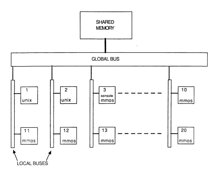
Fig. 2 Architecture of the Flex/32 Multiprocessor.
