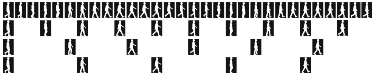
Fig. 2 Full period normalized silhouette sequences at various TRs from 85° view. The top row shows normalized silhouette sequences at 30 fps; the second row shows normalized silhouette sequences at 10 fps; the third row shows normalized silhouette sequences at 6 fps; and the bottom row shows normalized silhouette sequences at 5 fps. The silhouette sequences were taken from frame-skipped image sequences that started from the first frame
