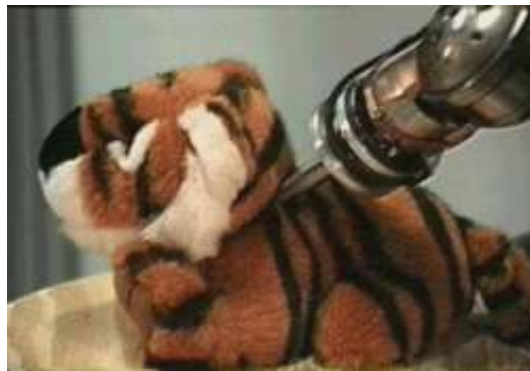
Figure 6.1: Robotic measurement of deformable objects: A stuffed tiger toy is being inspected by the force probe attached to ACME's Puma 260 robotic arm. The robot systematically contacts vertices of an associated multiresolution triangle mesh in order to measure displacement responses for related GFs. Stereo vision is used to measure surface movement during contact events.
