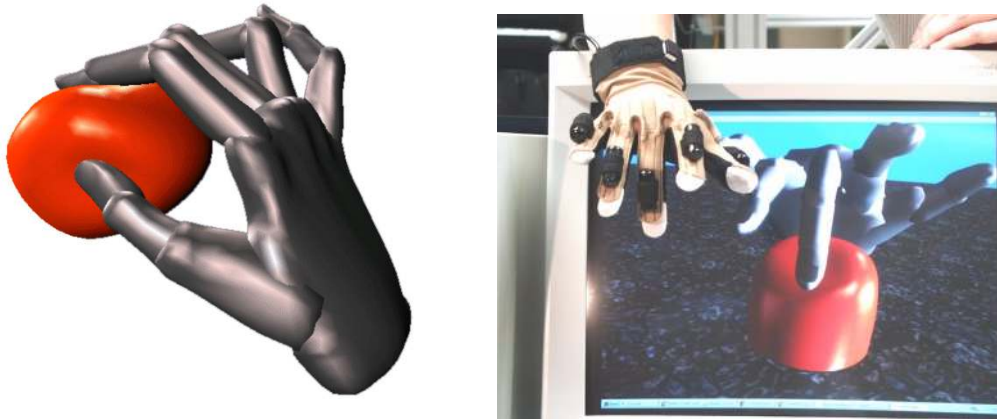
Figure 4.1: Interactive grasping simulation using a CyberGlove data input device (manufactured by Virtual Technologies Inc.). The virtual hand seen here was used to interactively deform a smooth elastostatic BEM model with approximately 900 surface degrees of freedom (dof) at graphical frame rates (30 frames per second) on a personal computer (dual Pentium II 450 MHz). The capacitance matrix algorithm was used to impose displacement constraints on an otherwise free boundary, often updating over 100 dof per frame. While force feedback was not present, this section shows how the capacitance matrices computed could also have been used to render contact forces at a rate much higher than that of the graphical simulation.
