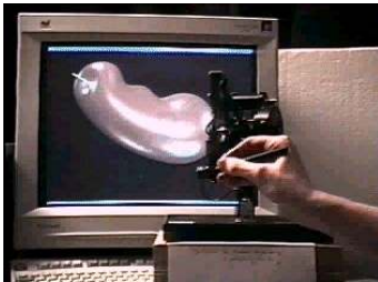
Figure 7.17: : Photograph of force feedback simulation in use : Users were able to push, slide and pull on the surface of the model using a point-like manipulandum. Additionally, it was possible to change the surface friction coefficient, as well as the properties of the pressure mask, with noticeable consequences. The PHANTOM™ (here model 1.0 Premium) was used in all force feedback simulations, and is clearly visible in the foreground.
