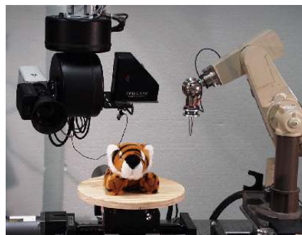
Figure 6.2: ACME Facility Overview: The UBC Active Measurement (ACME) Facility is a highly automated robotic measurement facility consisting of a variety of sensors and actuators, all under computer control.
