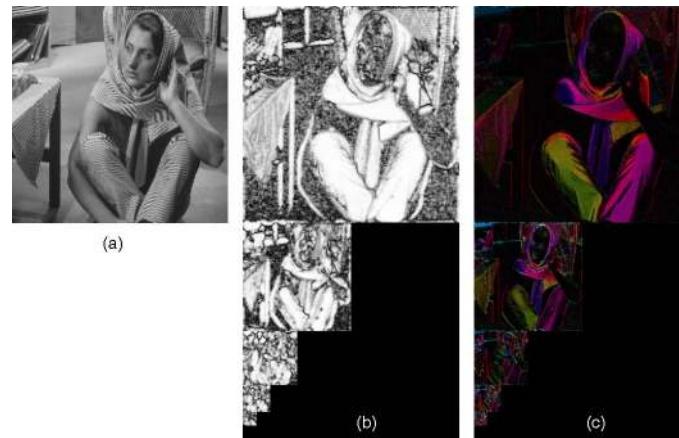
Fig. 9. Example of wavelet-domain coherence analysis. (a) 512 \times 512 Barbara; (b) wavelet-domain coherency map; (c) composite HSB display of results (Hue: orientation, Saturation: coherency, Brightness: amplitude).
