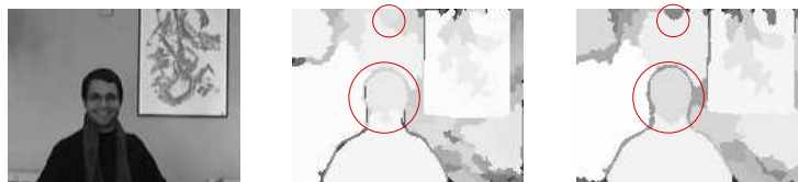
Fig. 6. Comparison of the effect of edge detection on the segmentation. Segmentation of the original image Sergi (top). Level of segmentation: \sigma_n = 25 pixels (left: not using edges, right: using edges).
