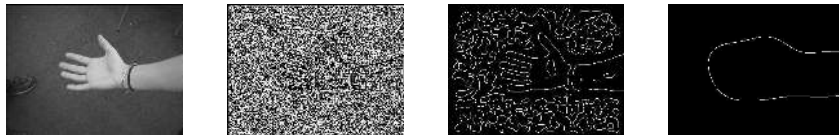
Fig. 4. Edge representation through scale using DOG (levels 1,4 and 7) and zero crossing detection. 1 sample per 3 octaves (first sample on the first octave)
