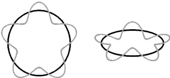
Figure 2: Left: The geometry \mathcal{S}_{i+1} (grey) is defined relative to the circle \mathcal{S}_i (black). For \mathbf{p} = [\cos(t), \sin(t)]^T \in \mathcal{S}_i we have \lambda(\mathbf{p}) = \frac{1}{4} \cos(5t) . Right: When deforming the base geometry \mathcal{S}_i \rightarrow \mathcal{S}'_i the modified geometry \mathcal{S}'_{i+1} is reconstructed by using the same detail function \lambda with respect to the new normal field N'_i on \mathcal{S}'_i . To evaluate \lambda at the correct location, the points on \mathcal{S}'_i and \mathcal{S}_i must be linked by a transformation map T .
