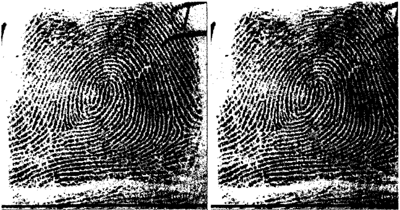
Fig. 16. Original and compressed image ‘fingerprints’, threshold 80, compression ratio 9:1, RMSE 25.50, L_1 error 20.17. Printed at scale 1:1 after histogram equalization.
