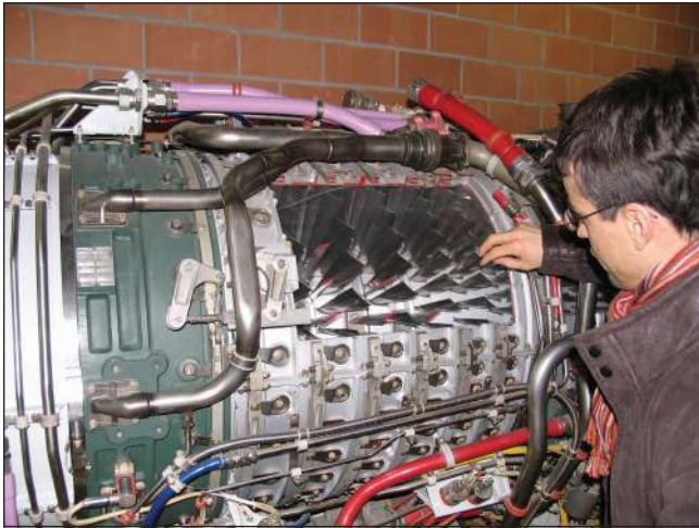
Figure 1. The compressor section of a jet turbine. The internal dimensions are within the same order of magnitude as those of the miniature robotic systems used in this article.
