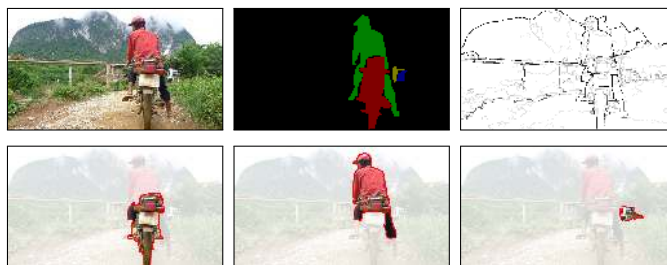
Fig. 1. Top : original image, instance-level ground truth from COCO and our multiscale hierarchical segmentation. Bottom : our best object proposals among 150.
