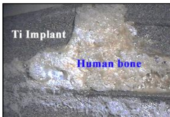
Figure I-2. Growth of human bone (osseointegration) on a plasma-sprayed titanium porous coating at 45 days after implantation (Courtesy of Hospital de Clínicas de Porto Alegre, POA, RS, Brazil).
