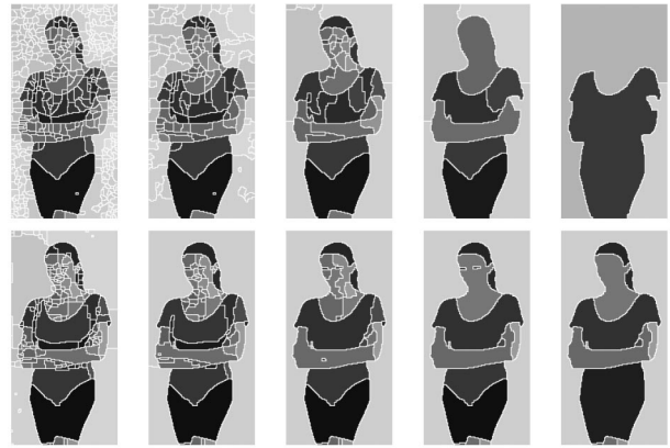
Fig. 5. Segmented scale-space stack after the projection of the regional minima. Top: Gaussian diffusion, from left to right: s = 0, 3, 9, 18, 31 with 456, 157, 43, 14, and 2 segments. Bottom: CLMC diffusion. s = 0, 5, 10, 15, 17 with 176, 71, 31, 16, and 13 segments.
