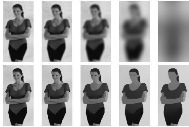
Fig. 2. Scale-space stack in YUV color-space. Top: Gaussian scale-space stack from left to right with s = 0, 3, 9, 18, 31 , \tau_o = 0.3 , and \delta\tau = 0.1 . Bottom: CLMC stack from left to right with s = 0, 5, 10, 15, 17 , \tau_o = 2.10 , and \delta\tau = 0.1 .
